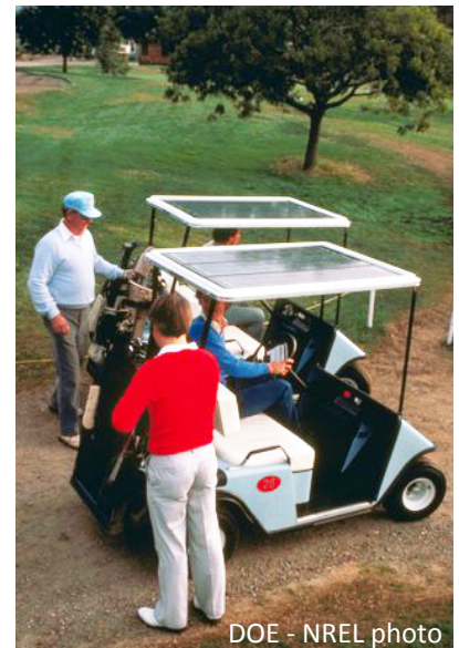
DOE - NREL photo The solar panels on these golf carts charge batteries that operate the carts.
